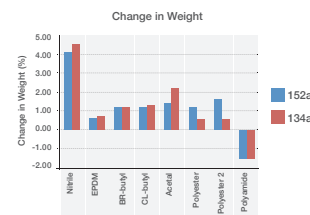
Figure 5 Changes in weight after propellant immersion (28-days 40°C)
